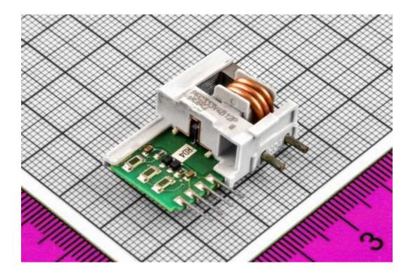
PFC333V4B12P is a type of current sensor produced by KOHSHIN in Japan. These sensors are used to measure electric current in different circuits.
